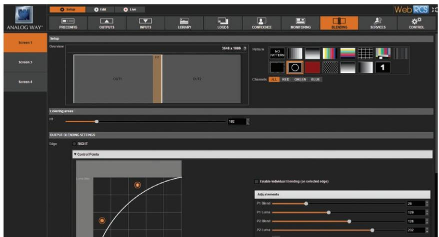
To setup an effective blend, you will first need to physically align the projected images so they are square with each other. Remember that you can adjust the number of lines and rows on the **LiveCore™** grid test pattern. to assist you.
