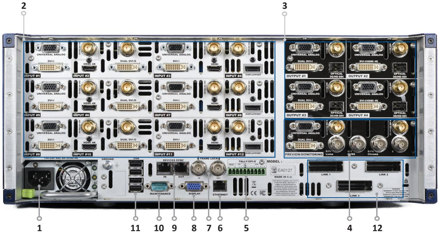
**1. Power supply:** internal, autoswitching ; Typical consumption: **Ascender 48:** 405W / **Ascender 32:** 345W / **Ascender 16:** 285W / **SmartMatrix Ultra:** 285W ;
