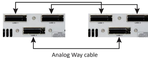
**Associative Modularity mode** allows for up to four units to be used as part of the same Assembly on the Vertige™ console. The Device Sync connection assists with synchronization between the various units. In Associative Modularity configuration, video information must be externally split and shared with all devices in the Assembly.
