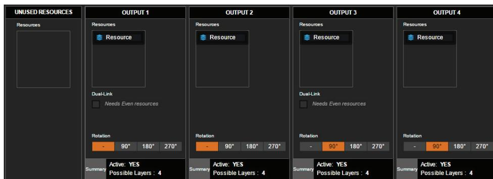
The Outputs section defines if you use any of the outputs in Dual Link or 4k modes, or if you reassign the layer resources of an output to another one. To activate a Dual Link output, drag the adjacent resources onto output #1 or #3, then check the Dual Link option box.
