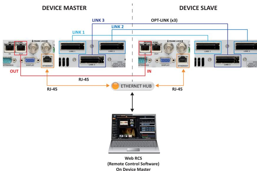
Once the two devices are wired up, ensure that all devices have unique IP addresses on the network, and that the gateway IP of all devices is set correctly. If you are not using a router on the network, set all of the gateway IP addresses to the first or last IP on the network, for example 192.168.2.1 and do not use this address for any other device.
