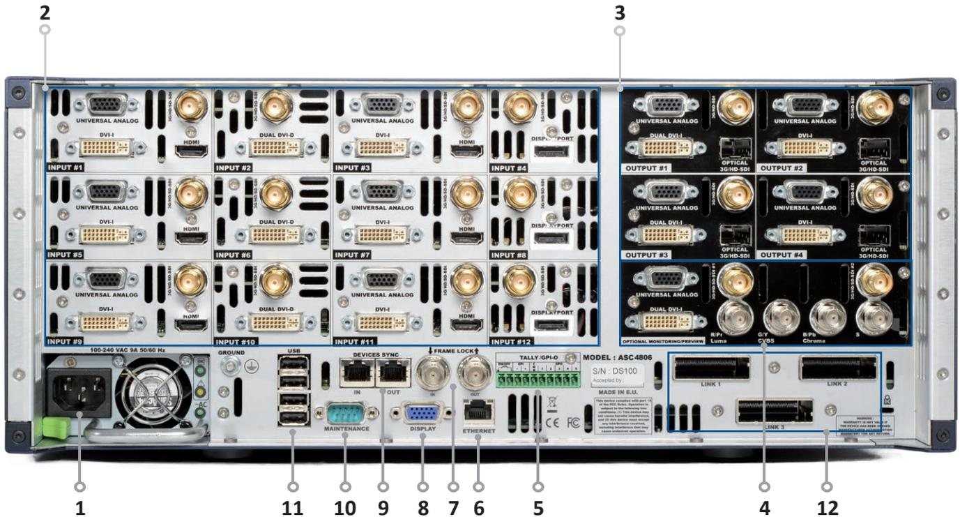
**1. Power supply:** internal, autoswitching ; Typical consumption: **Ascender 48:** 405W / **Ascender 32:** 345W / **Ascender 16:** 285W / **SmartMatrix Ultra:** 285W ;
