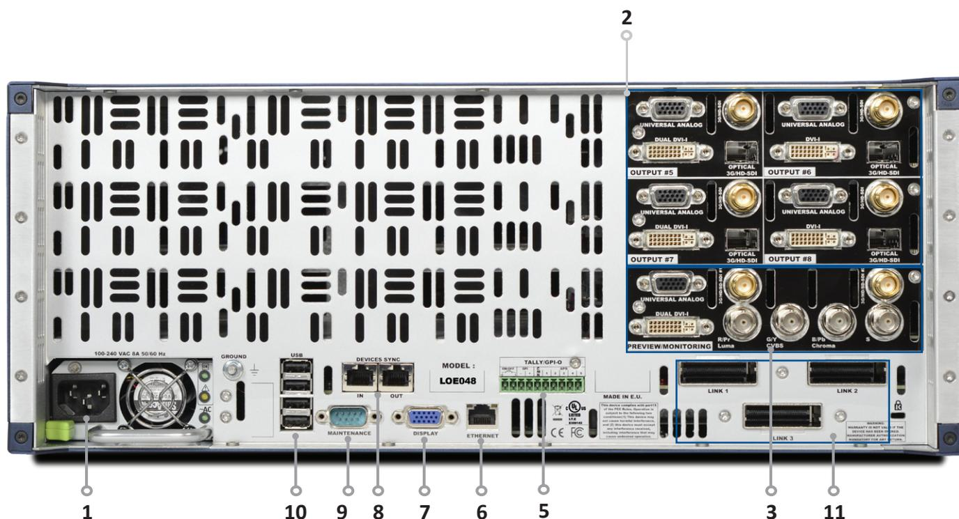
**1. Power supply:** internal, autoswitching ; Typical consumption: 405W
