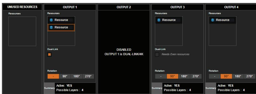
To activate an output for 4k resolutions via HDMI 1.4 (on units with the 4k hardware option), drag the adjacent resources to outputs #2 or #4 and then check the «4k» option box.
