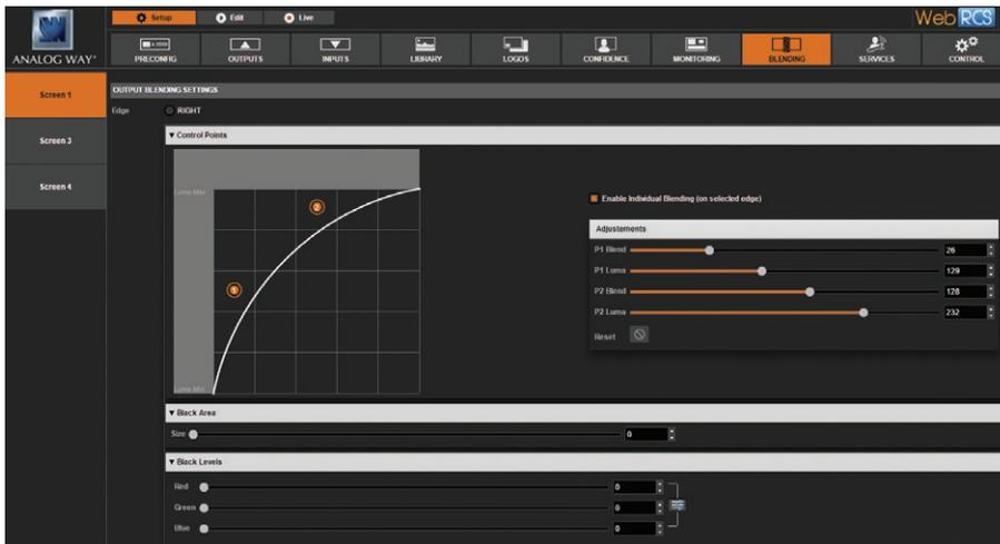
Click on the left/right side into the overview of your Soft Edge, some settings appear. Then adjust the black levels for each side using the R,G,B level to make each non-overlapping part of the projection as bright as the overlap zone.
