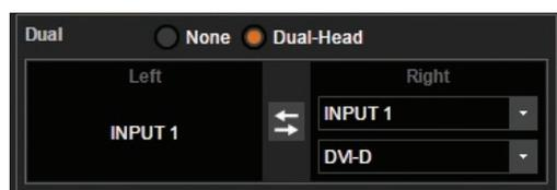
Under the Input setup menu, you can check the feature **DUAL-HEAD** of your inputs. You just need to indicate which second plug is linked to the actual input. In this example, the input #2 is linked in Dual-Head with the input #1 .
